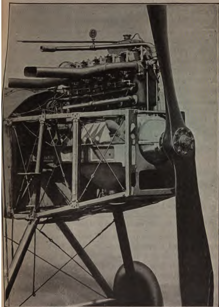
Fig. 77. Installation of Direct Driven Tractor Screw Which Turns at Engine Speed.
